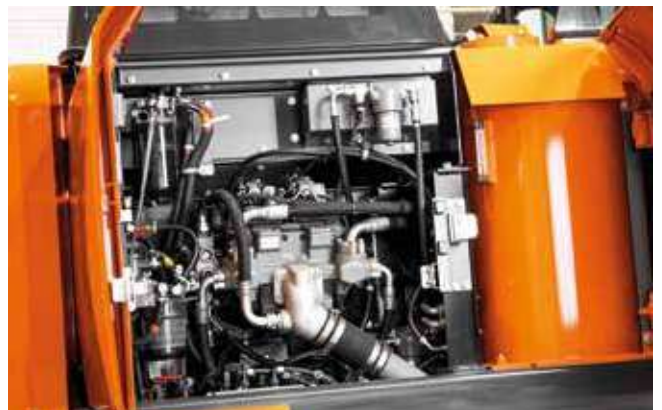
The HIOS III hydraulic system contributes to significant reductions in fuel consumption.
