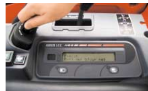
2 Insert new individual Black operational key
