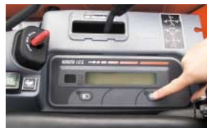
1 Insert the Red programming key, then press the monitor button
