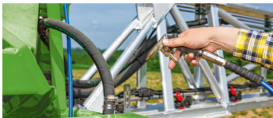
□ The optional compressed air gun is situated at the back on the boom for quick cleaning.
