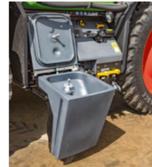
The lowerable induction hopper for ergonomic operation and easy filling.
