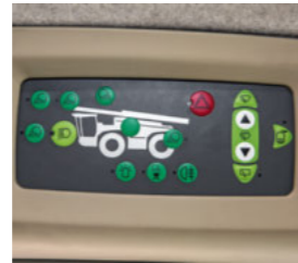
■ Single or shared switch for work lights.
