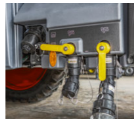
□ Hydrant filling connection with return valve.
