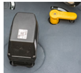
■ OptiFlow control centre: Arranged alongside the induction hopper for easy control of all agitators and filling functions during the filling process.
