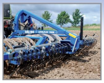
The front mounting and improved geometry pull the packer forwards, making it easier to control.
