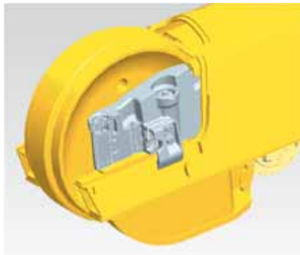
Self-adjusting idler support
