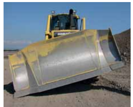
Hydraulically adjustable tilt: 870 mm
